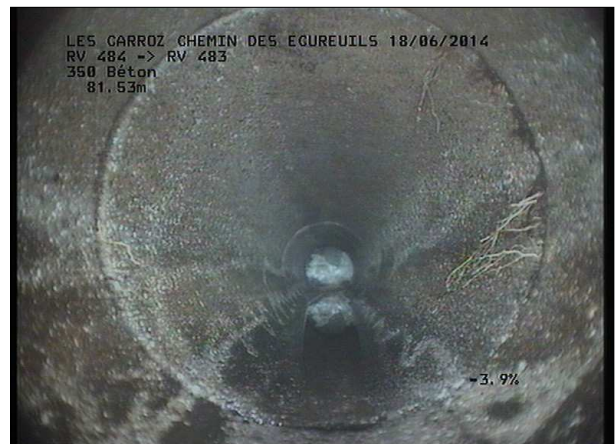
Photo: 23_21A, MPEG #: 160614_1, 00:13:54 81,77m, Radicelles de 12 à 12 h.
