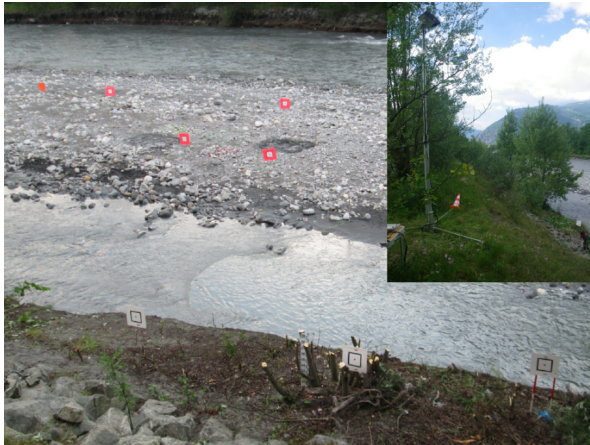
Figure 3. Photo of the set-up for video analysis showing GRPs (photo inserted: mast on which the camera is fixed).
